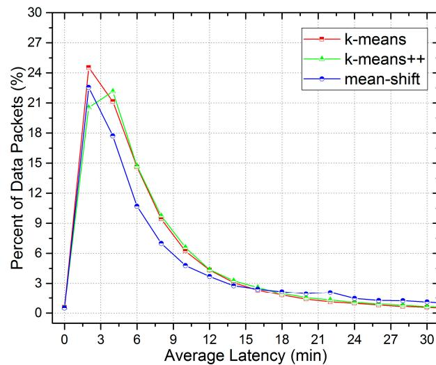
**Figure 9.** Distribution based on the latency of uploaded data packets.
